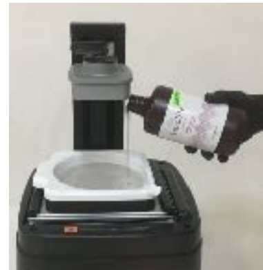
Adding liquid Vitrolite to printer
