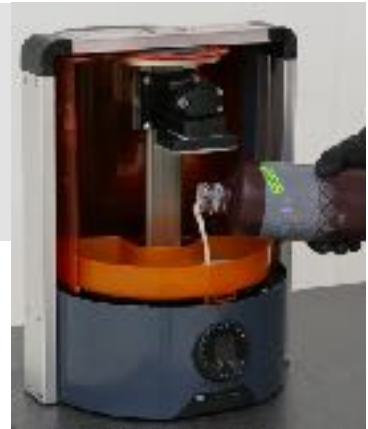
Adding liquid Porcelite to printer
