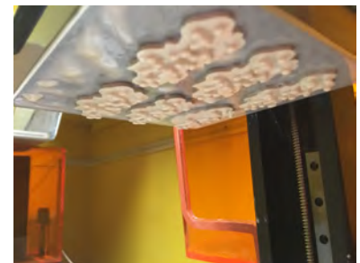
Pausing a printer to check for adherence
