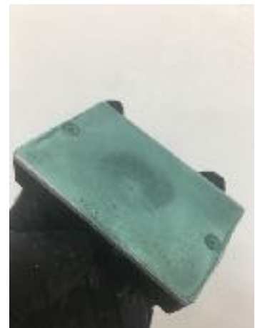
Apply a Polyester adhesive backed film for easy part removal
